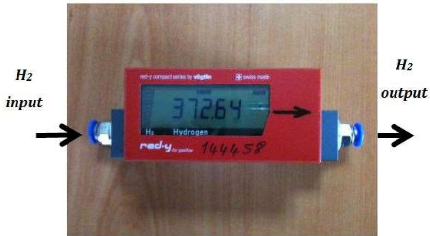
Figure 16. Connection of the H 2 flow meter in the gas flow direction
