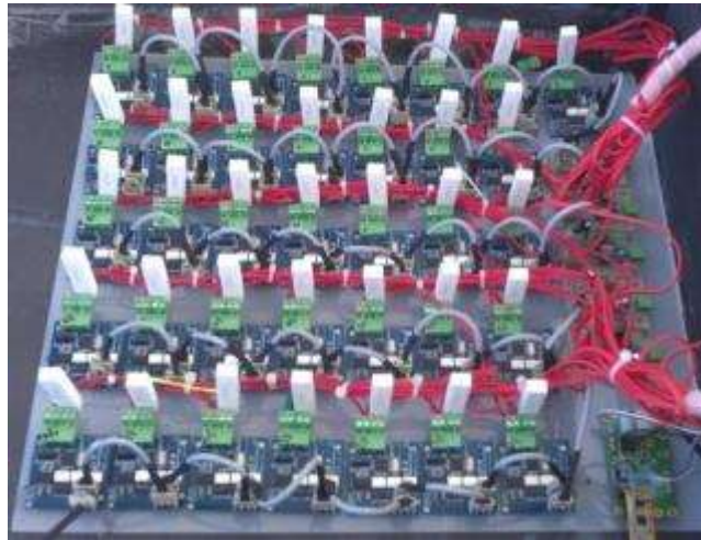
Figure 8-b. Sample BMS for lithium-based batteries
